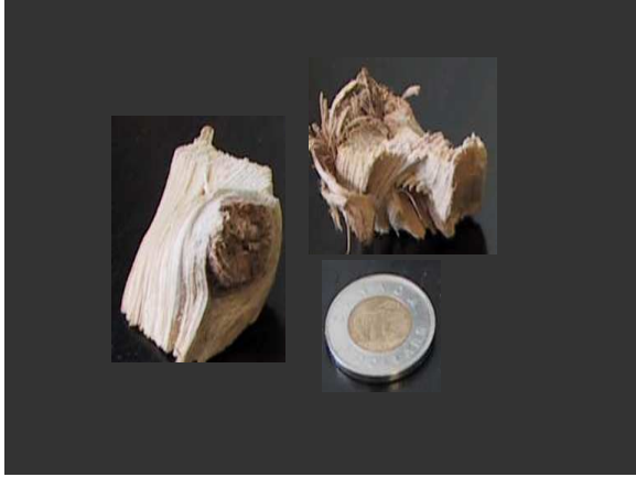
Figure 1. Biological wood knots are derived from chipping a part of a tree stem into which a branch was sticking. Their cores tend to be round in cross-section, higher in density than normal stem wood from the same tree, darker in colour, and more heavily lignified. Knots are surrounded by reaction wood, which is also different from stem wood. (The twoonie is 28 mm in diameter).
